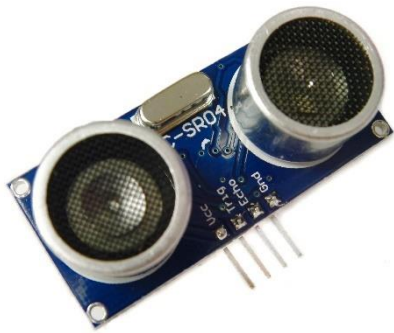
Figure 5.16 - Hc-Sr04 sensor and Ultrasonic sensor connected to Rapsberry pi
